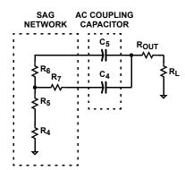
FIGURE 4. SAG NETWORK AND AC COUPLING CAPACITORS
